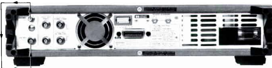
Figure 4.2. HP 11729C cable hookup for 640 MHz self-generation.
